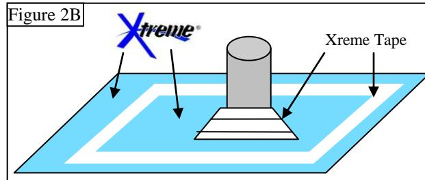
Note: For maximum adhesion of the tape, apply the Xtreme Tape immediately after the Tex-Trude Xtreme Vapor Barrier Patch has been placed. The area should be free from dirt, dust, and moisture.
