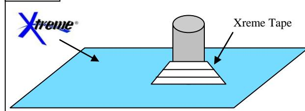
2. Larger spaces around pipe: Cut a piece of Xtreme in a shape, larger than the repair, insuring a minimum six inch overlap in all directions and tape all of the edges. Cut an X the size of the pipe or slightly smaller for a snug fit and slide the patch over the pipe and seal the pipe with the Xtreme Tape. ( See figure 2A, 2B )
