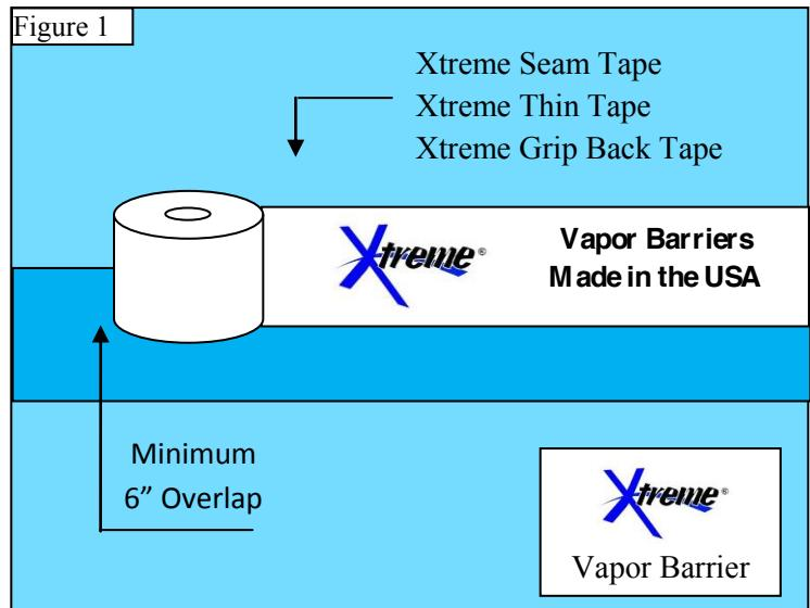
Note: For maximum adhesion of the tape, apply the Xtreme tape immediately after the Tex-Trude Xtreme Vapor Barrier has been placed. The area should be free from dirt, dust, and moisture.
