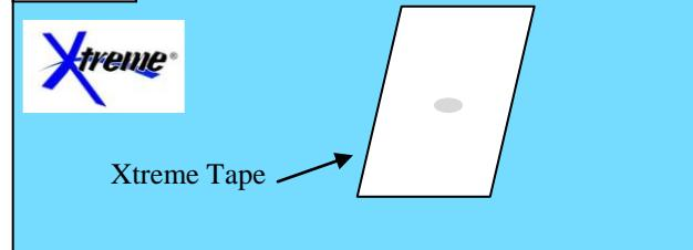
2. Larger Repairs –Cut a piece of Xtreme in a shape, larger than the repair, insuring a minimum six inch overlap in all directions and tape all of the edges. (See figures 2A, 2B, 2C)
