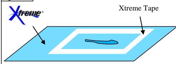
Note: For maximum adhesion of the tape, apply the Xtreme Tape immediately after the repair has been placed. The area should be free from dirt, dust, and moisture.
